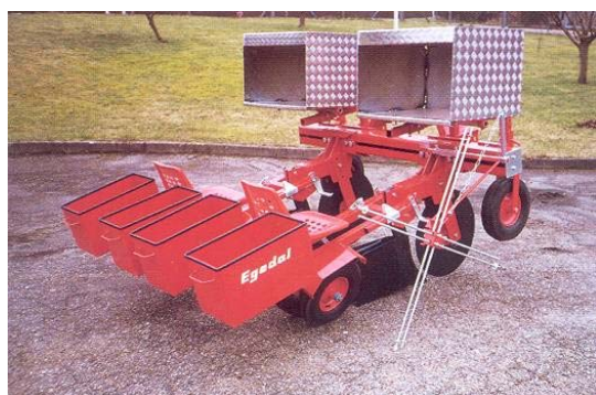
Two-seater transplanter available with all weather cap, furrow marker, electronic distance marker, spot fertilizer and boxes for sticks
