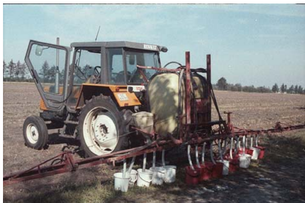
Calibration of juice spreader. The distribution of juice is checked before and after application on each plot
