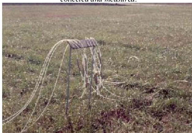
Vacuum probes with thin plastic tubes connected through the top stopper. The leaching of nutrients is monitored for each plot every week over a three-year period.
