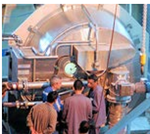
Peeler centrifuge applied in cornstarch dewatering.
