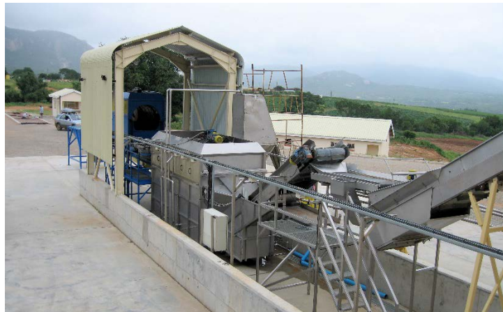
Intake and washing 20 t/h of fresh cassava roots
