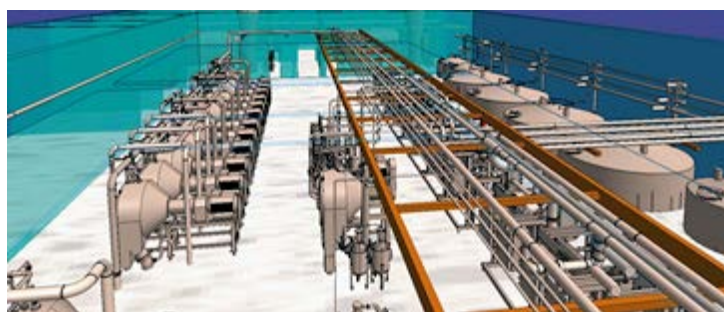
Refining section. Centrifugal screens left. Hydrocyclones right.
